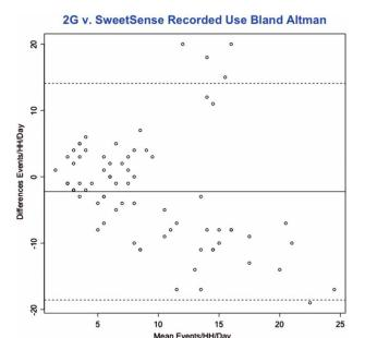
Figure 1 | Bland Altman Test: 2G PLUMs versus SweetSense PLUMs recorded use
